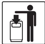
Make the appliance unusable by removing the power cable and any compartment or cavity closing mechanisms (when present) in order to avoid the risk of someone becoming closed inside.
